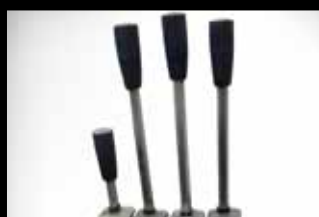
Four in-cab cable control levers (or electro-hydraulic controls).
