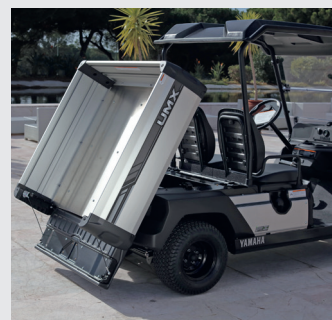
Aluminium cargo bed with one-touch tailgate.
