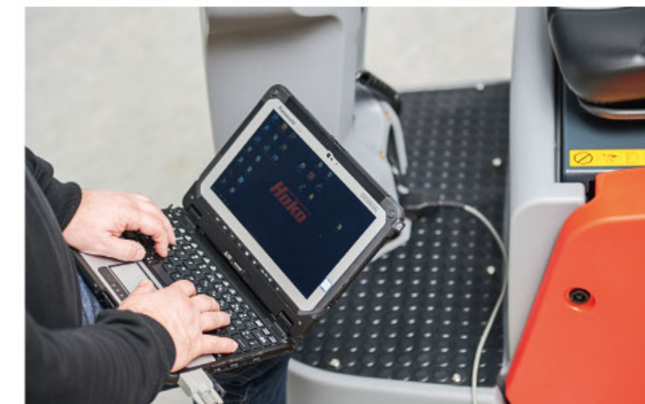
Easy access to the diagnosis interface allows both easy maintenance and modifications to the driving settings.
