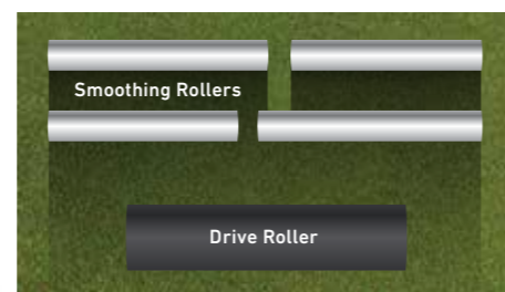
Offset smoothing roller design for uniform greens appearance and playability
