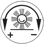
Wear compensator for rotary brush (Fig. 2/3)
